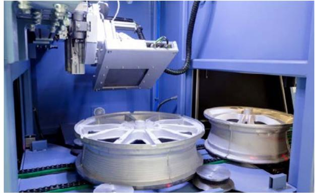
The system is able to operate with different designs and sizes of wheels coming randomly from the production platforms.
